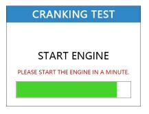
After entering the second start system test function ,the press OK key as following:Starting the engine as prompted, tester will automatically complete the cranking test and display the result.
