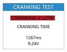
If the engine starting can't be detected, there may be no output of charging voltage, you need to check the generator.
