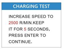
Tester starts the charging volt test after increase rev detected.
