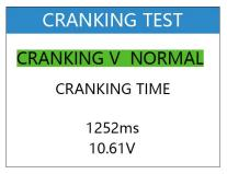
When cranking test is abnormal, battery test result will also be displayed at the same time. This is for the convenience of the maintenance personnel to quickly know the whole state of the starting system according to the data.
