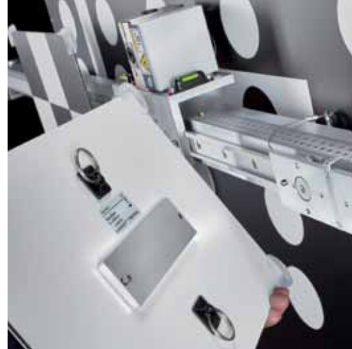
Just plug the targets onto the precision slider using the magnetic clamps
